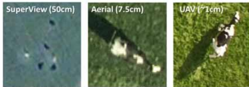
Figure 2 Cow visibility on different platform imagery. Left to right: SuperView VHR satellite imagery (50cm), Aerial (7.5cm) and UAV (~1cm).
